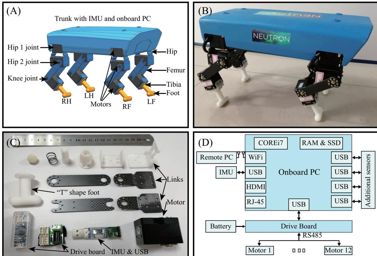
**Figure 3.** Lilibot. (A) CAD model. (B) Real robot with a weight of 2.5 kg. Its length, width, and height are 30 cm, 17.5 cm, and 20 cm, respectively, when it stands. (C) Main components of one leg. (D) Mobile processor system.
