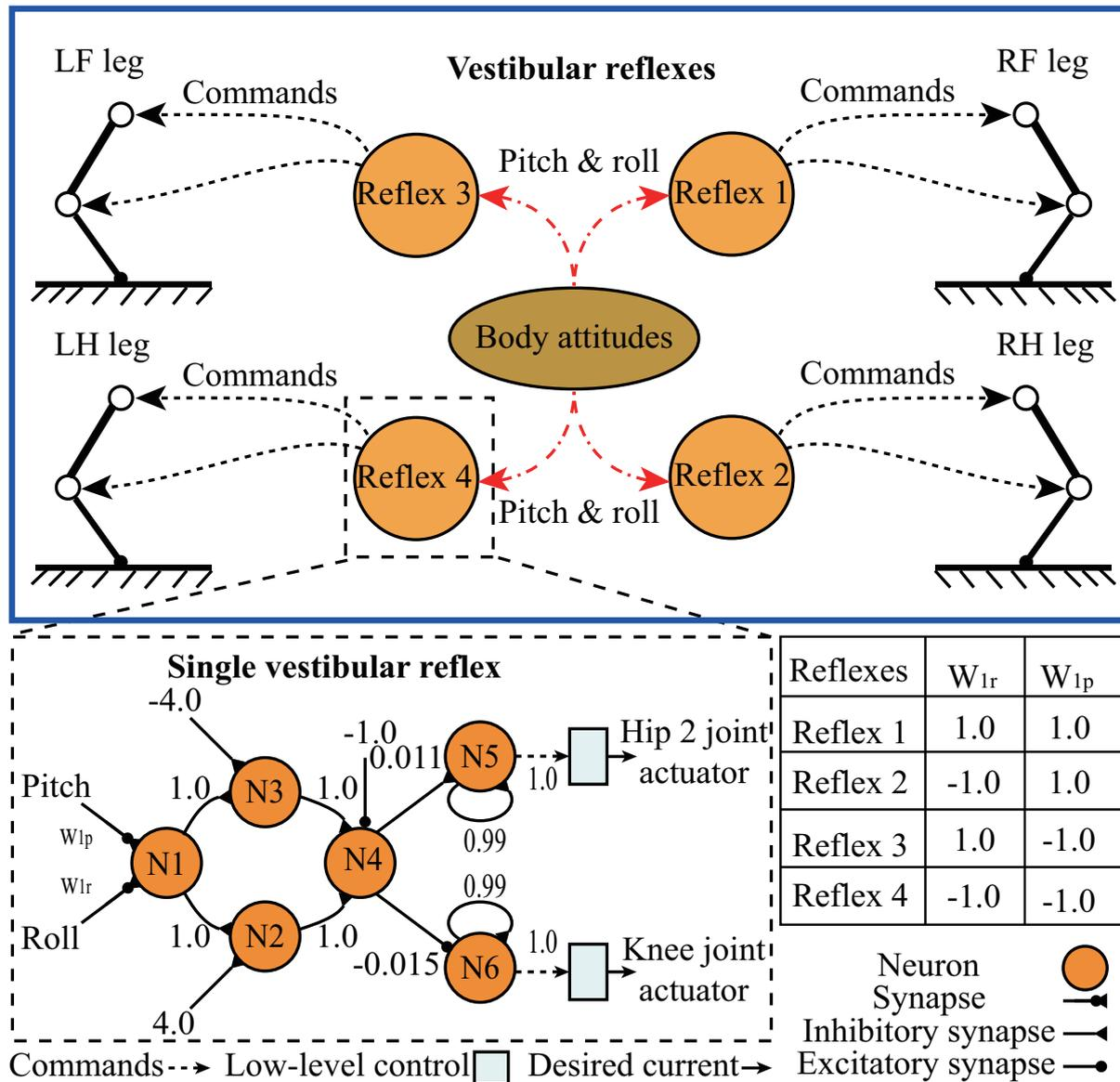
**Figure 7.** Schematic of vestibular reflex control mechanism. The weights of the neural reflex network are set empirically.
