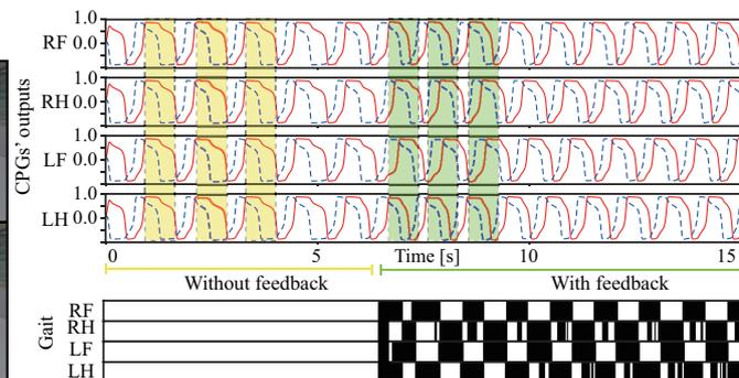
**Figure 9.** Process of self-organized locomotion generation under four leg orientation types. The outputs of the CPGs started in phase, and once the robot interacted with the ground, the phases began to be adjusted by the GRFs. The gaits quickly emerged within 8 s.
