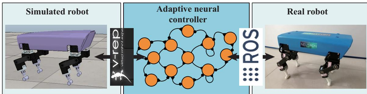
**Figure 1.** System overview of Lilibot. The adaptive neural controller is implemented in ROS such that it can directly communicate with both the simulated robot in the V-REP simulation and the real robot. The simulated and real robots were consistently developed, such that the simulation demonstrates a good estimation of the actual performance. A video showing a comparison between the simulated and real robot behaviors can be seen at <http://www.manoonpong.com/Lilibot/video6.mp4>.
