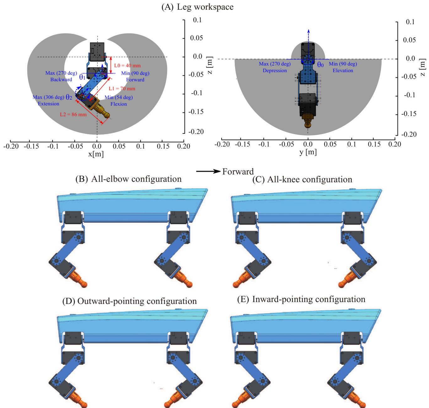
**Figure 4.** Leg workspace and various configurations. (A) The leg has a large and symmetric workspace that enables the robot to exhibit four different configurations or orientations, as indicated in (B) to (E). (B) All-elbow configuration. (C) All-knee configuration. (D) Outward-pointing configuration. (E) Inward-pointing configuration.
