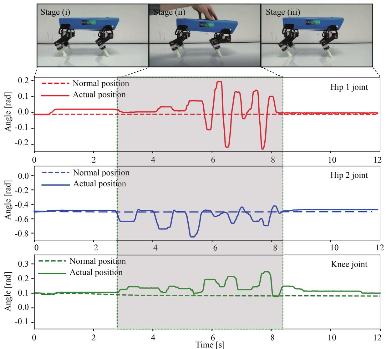
**Figure 10.** Compliant behavior of Lilibot and angle feedback of the hip 1, hip 2, and knee joints of the RF leg. The normal positions of joints were the desired positions of compliant control. The robot was placed on the ground and was standing in the initial stage (i). In stage (ii), a hand was used to apply a force on its body, and the robot exhibited compliance to compensate for the perturbation. During stage (iii), the robot returned to its normal position after the load was removed.
