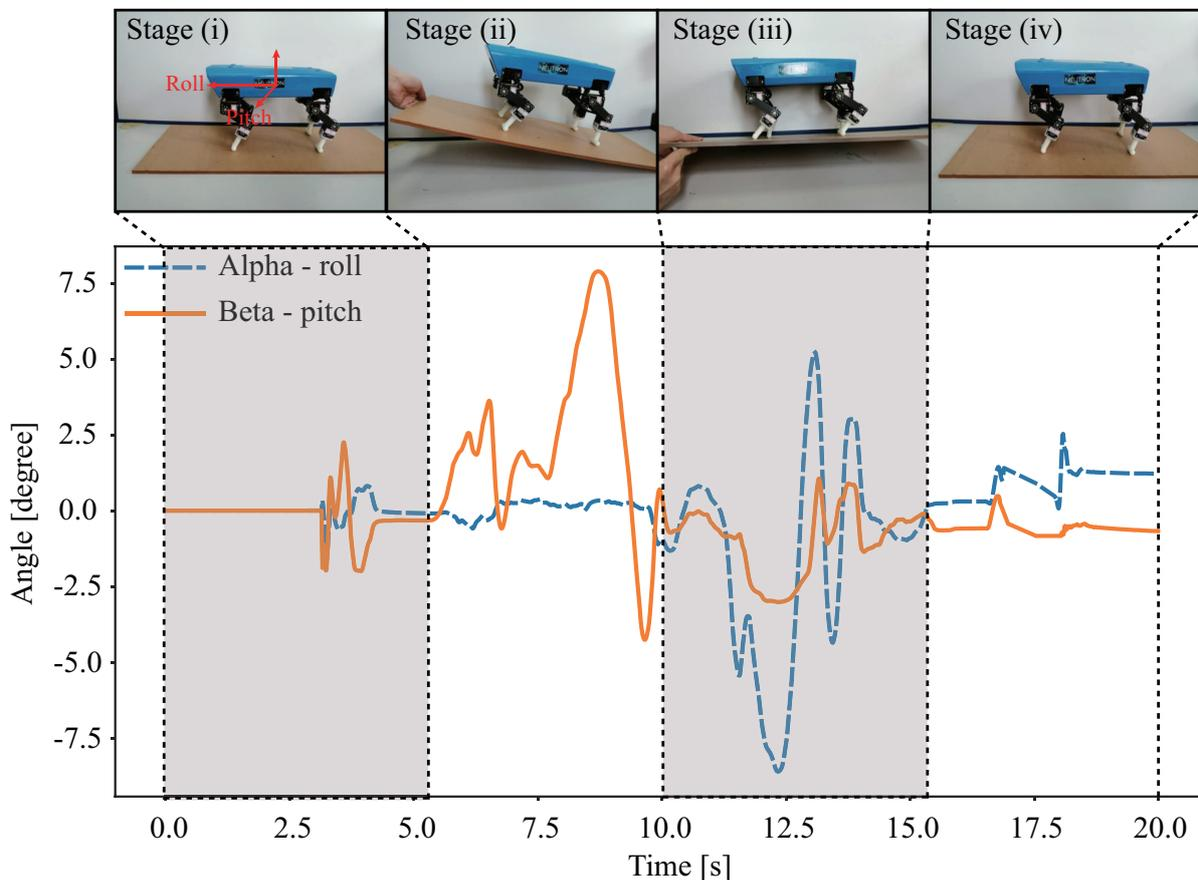
**Figure 11.** Snapshot and body attitude angles of Lilibot in the experiment, where Lilibot sustained its body attitude stabilization while the supported tiltable plane inclined around the pitch and roll planes in stages (ii) and (iii), respectively.
