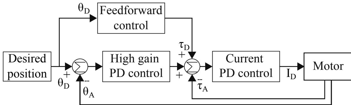
**Figure 8.** Block diagram of compliant control mechanism loop:  $\theta_D$  and  $\theta_A$  represent the desired and actual joint positions, respectively;  $\tau_D$  and  $\tau_A$  are the desired and actual motor torques; and  $I_D$  is the desired current for driving the motor.
